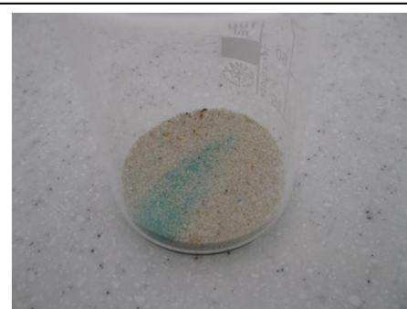
The malechite rock is finely crushed before processing. Explain why this is necessary.
